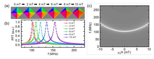
**Figure 3.** (a) Simulated domain structures of the magnetic vortex under various external magnetic fields. (b) Field dependence of the FFT spectra under the partial positive magnetic fields. (c) Image plot of the FFT spectra under the external magnetic from -10.0 mT to 10.0 mT.
