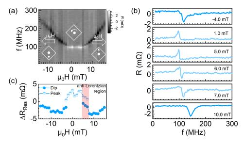
**Figure 2.** (a) The image plot of frequency dependent spectra with sweeping the external magnetic field. The vortex core displacement is also shown with counterclockwise chirality. (b) Magnetoresistance spectra with specific external magnetic fields. (c)  $\Delta R_{\text{Res}}$  as a function of the magnetic fields. The blue and light blue dots stand for the resonant dip and peak, respectively.
