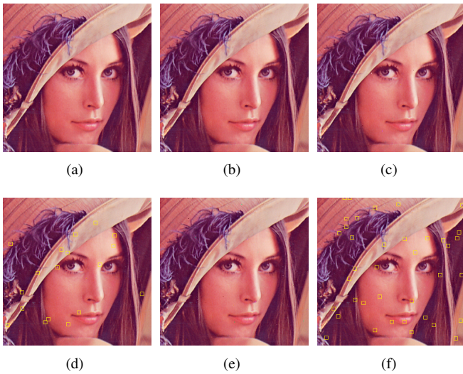
Fig. 10. Image quality comparison using 'Lena' image among different bit error rates: (a) 1 \times 10^{-6} , (b) 1 \times 10^{-5} , (c) 5 \times 10^{-5} , (d) 5 \times 10^{-5} with error tag, (e) 1 \times 10^{-4} , and (f) 1 \times 10^{-4} with error tag.
